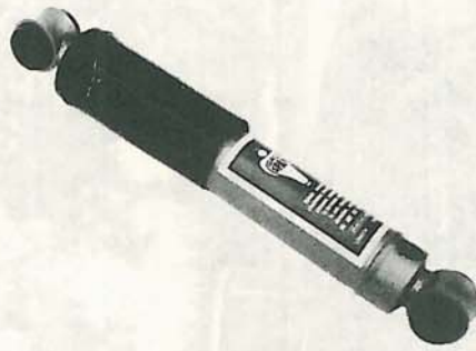
A Spax adjustable telescopic damper for the front end of a Spitfire/GT6. These come with all necessary mounting rubbers and can be combined with uprated springs as desired.
