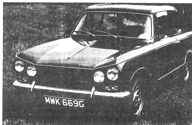
Slight changes to the grille, false "Rostyle" wheel covers, and radial ply tyres are recognition points, but there are no styling changes to metal pressings
