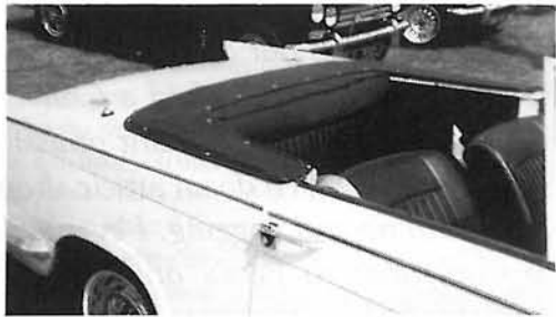
Figure 7 - Fit the hood cover or tonneau. This should lie flat with no bumps if the roof has been folded properly.
