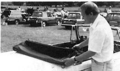
Figure 4 - Pull the windscreen rail upwards with one hand, whilst pulling the excess roof material over the second rail, outwards with the other hand.
