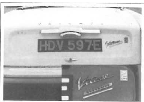
Figure 15 - The rear of the 2-Litre Mk.1. The number plate bezel is cut out to accommodate a combined number plate light and reversing light. The inset shows the correct position of the 2-Litre Mk.1 overdrive badge.
