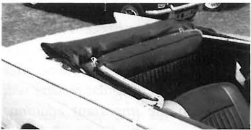
Figure 5 - Fold the frame into the hoodwell, tidying away the clips and laying the excess roof material on the rear deck.
