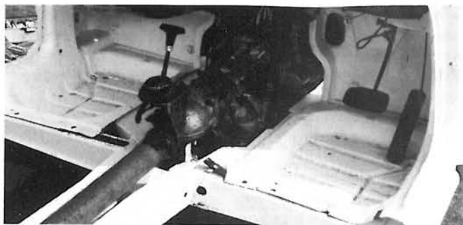
Bulkhead meets chassis! Note the lack of clutch pedal
