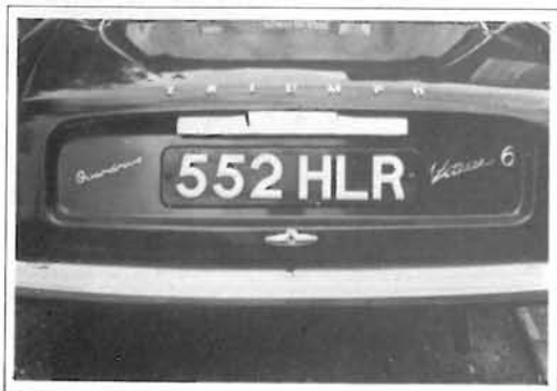
Figure 14 - Badges on the rear of the 1600. Note the correct position of the optional overdrive badge.
