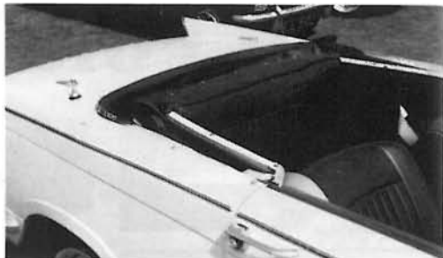
Figure 6 - Fold the excess roof material tidily over the frame.
