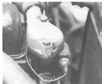
Figure 32 - 1600's up to engine nos. HB 27,986 were fitted with water pump housings with a single tapping for the temperature sender unit.
