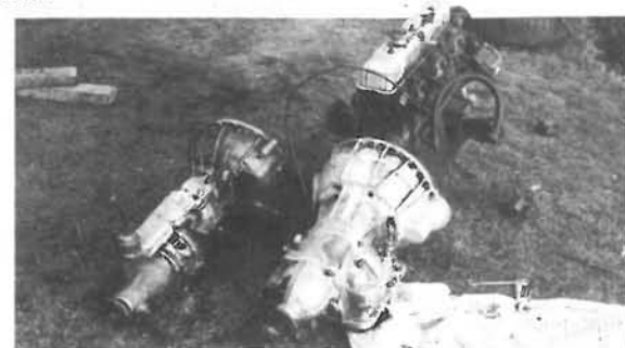
Automatic gearbox mated to engine with manual alongside
