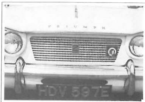
Figure 13 - On the 2-Litre Mk.1, the grill remains the same but a 2-Litre badge is added. The Triumph badge is deleted. A smaller 2-Litre badge is fitted above the bonnet catches on either side of the bonnet.
