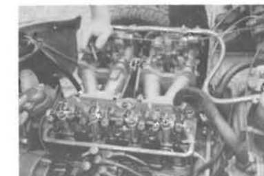
Gleaming Rockers. Note direct oil pipe to rocker shaft oil feed line -bottom right.
