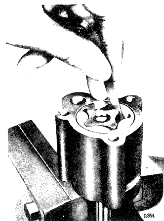
Measuring clearance between inner and outer rotors
