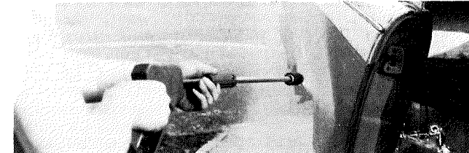
Fig: 5 - As you can see, the pressure of the jet causes a lot of bounce back overspray so be prepared to get wet! Nozzle pressures range from about 40 to over 600psi depending on the lance nozzle settings. Unlike as shown in the photo, keep all mains cables well out of the line of fire.
