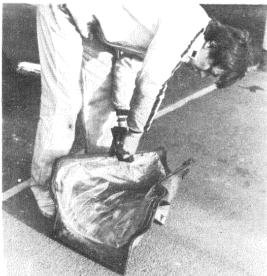
FIG. 31: The sound deadening 'parcel' on my gearbox cover was absolutely ripped to bits, so we reparcelled it up with fresh polythene - as good as new. Here Bernard's tacking the restored lining back on.
