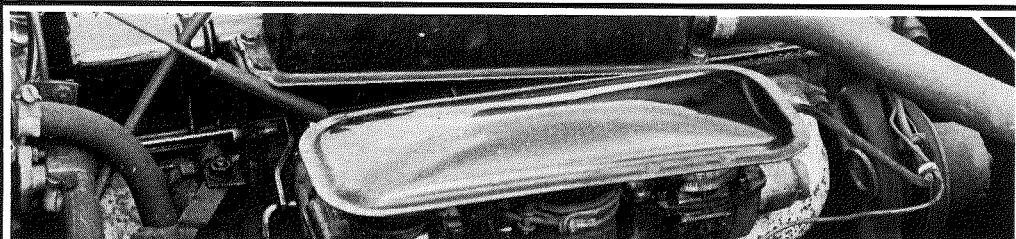
Early Vitesse 6 engine showing fitment of downdraught Solex B321H carbs - note: also early type radiator with separate header tank fitted from HB6798E to 27985E
