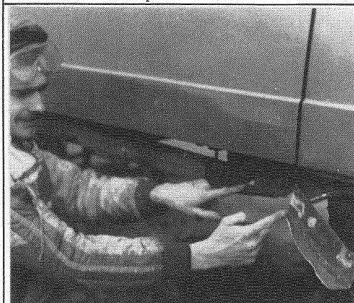
Plate brazed over holed chassis and then floor pan - Ughh!
