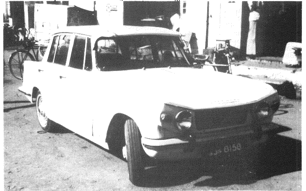
FIG. 2 Standard Herald MKII Four-door saloon version with integral sidelight/indicator (photo Mike Long)
