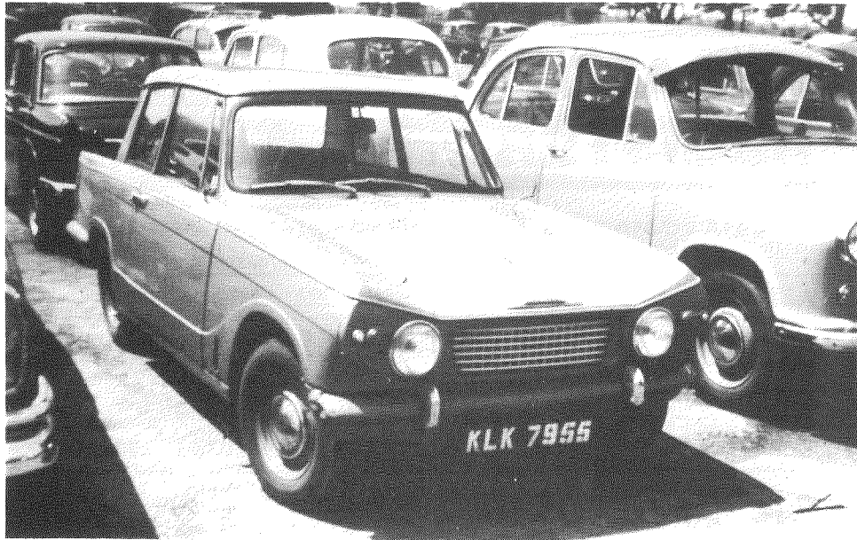
FIG. 3 Standard Herald MKII Two-door version with separate sidelights and indicators. (photo Mike Long)
