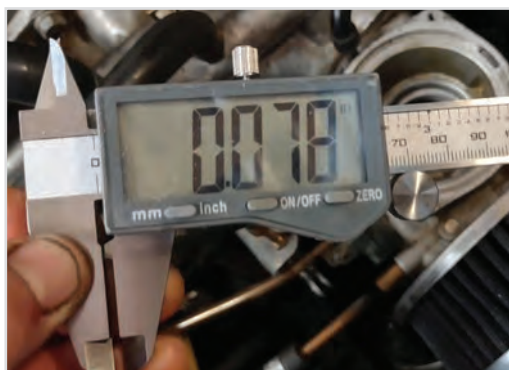
Front Carb Jet depth was 78 thou
