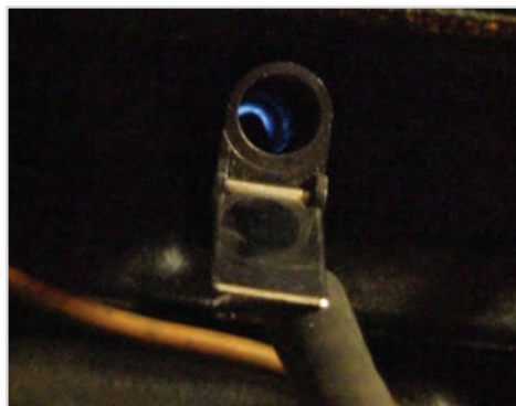
Checking the mixture with a Gunson's Colourtune
