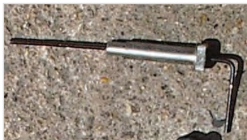
Stromberg CDSE mixture adjustment tool
