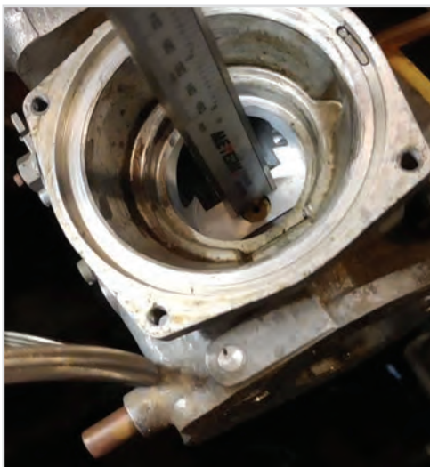
Checking the jet depth below the bridge with a digital vernier calliper
