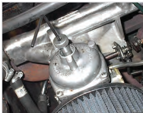
Using the adjustment tool to set the mixture by adjusting the height of the metering needle
