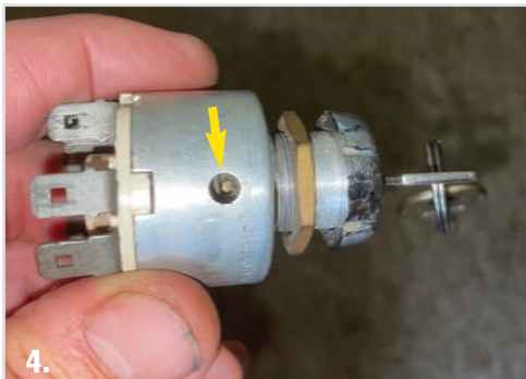
Ignition drum – showing access hole and brass button.
