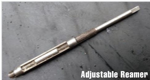
Reaming Carb bodies for New Spindles
