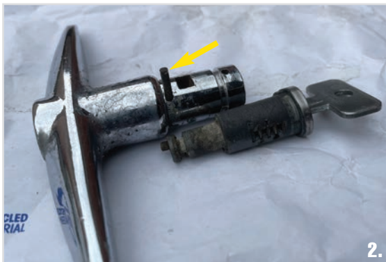
Boot Handle showing pin to extract to enable lock barrel removal
