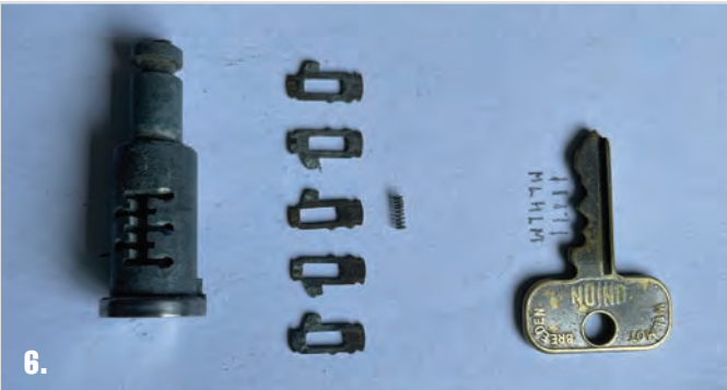
Boot Lock barrel with blades removed – one loose spring
