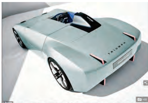
The single-seat roadster is powered by a rear-mounted 184bhp electric motor sending drive to the rear wheels only. It is claimed to be able to hit 62mph from a standstill in just 5.2 seconds
