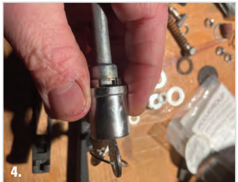
4. Lock Actuator Barrel with Spring removed
