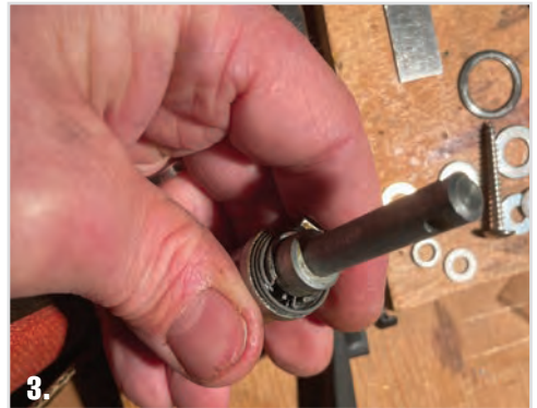
3. Lock Actuator Barrel showing Spring position
