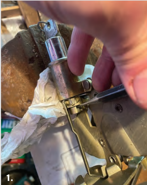
1. Early door lock – extracting clevis pin to withdraw lock actuator.
