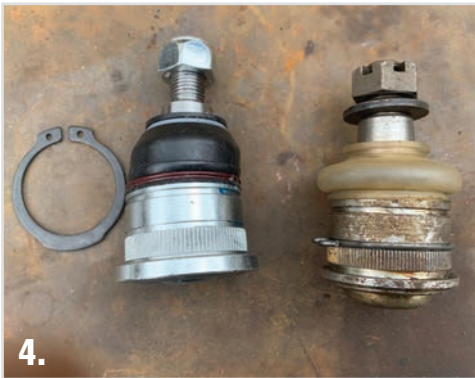
Pic No. 4 shows the new joint that I now use these have been extensively tested and used on my own cars with no issues. Another bonus of these is they have a correct profiled boot that keeps the water out and doesn't require it to be removed for fitting.
