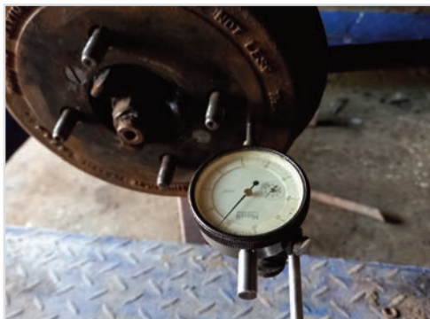
Checking Brake drum Run out
