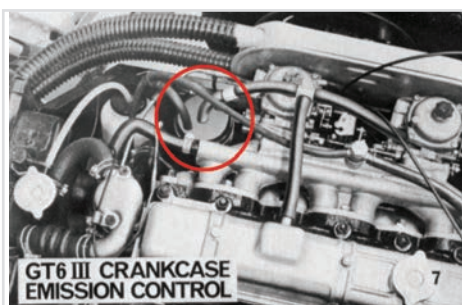
Carburettor Evaporative Breather Canister, part of emission control system
