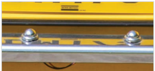
US Export number plate lights at side of number plate.
