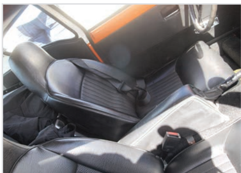
High Back Seats Fitted to US, Japan and Australia export models (up until the separate headrests became standard in late GT6 MK3 swing spring models).
