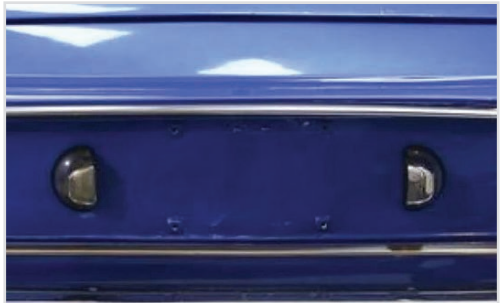
US Export number plate lights at side of number plate.
