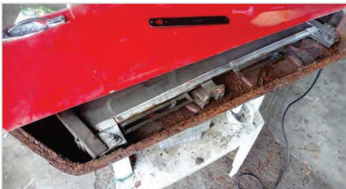
New door Frame Bottom needed
