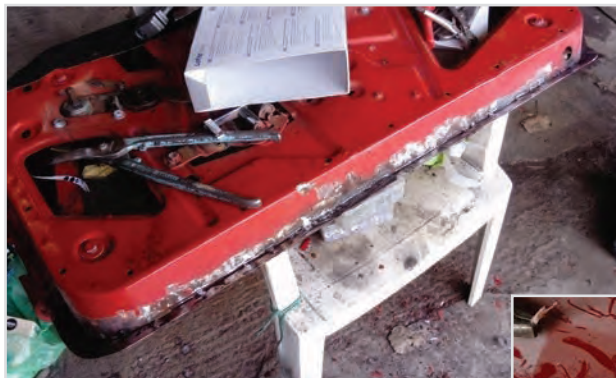
Door Frame Repair Sections welded in place
