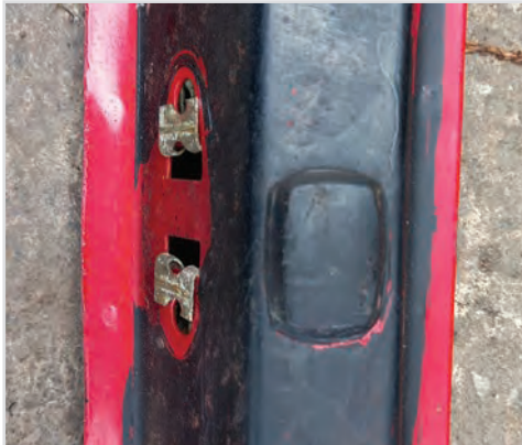
Blanking Rubbers over the Spit Frame Spire Nut Holes
