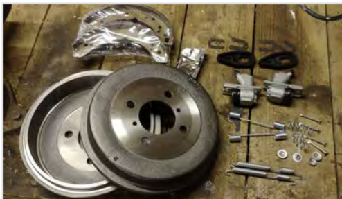
Brake overhaul parts sitting ready for replacement on my GT6.
