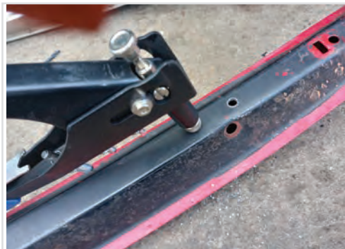
Threaded Rivets being Fitted
