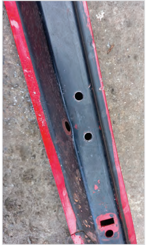
Holes Drilled for Clasp Fittings
