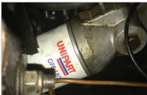
Spin on conversion with Oil Filter connections as fitted to my GT6
