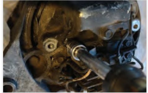
Remove the screw securing the earth fly lead from the regulator, this is also one of the securing screws for the brushbox
