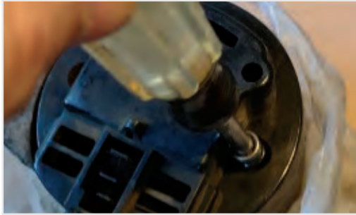
Removing the hex headed screws securing the cover
