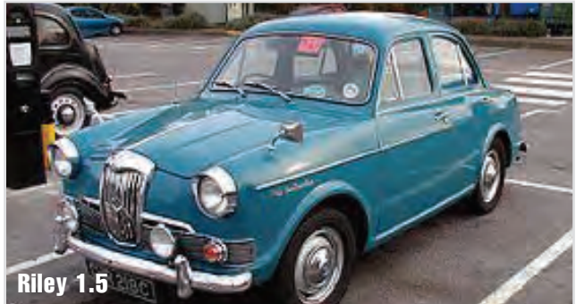
My first car was a BMC Riley One-Point-Five with the 1489cc 'B' series. This one had the MGA, MGZA and ZB cylinder head
