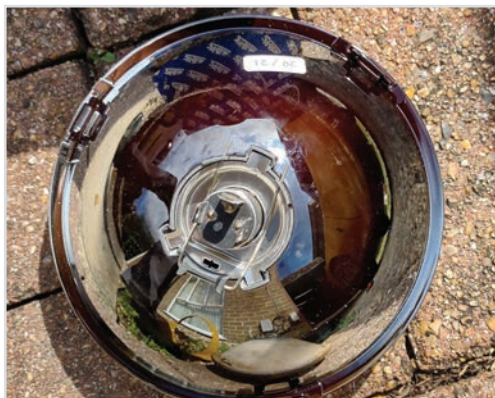
The Halogen Bulb fitted in place held with a spring clip
