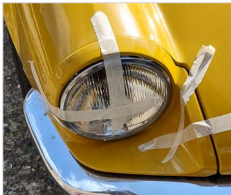
Temporarily holding the cowl in place with masking tape.
