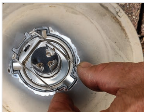
Removing a halogen bulb
