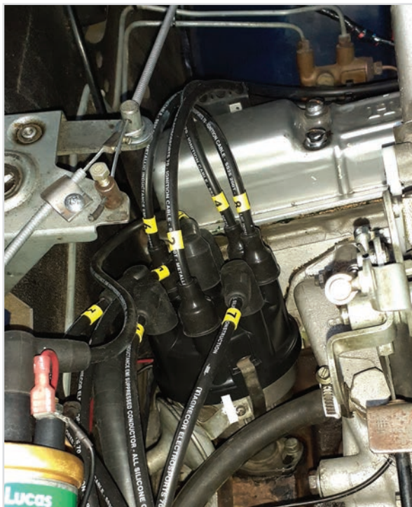
Pic 3. Magnecor leads and new cap
