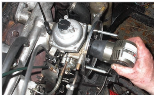
Tuning the carbs, adjusting the balance
