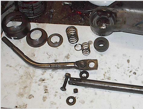
Gear Lever and remote strip down for overhaul
