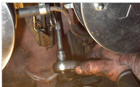
Tightening Manifold Bolts with a universal socket coupling and extension
