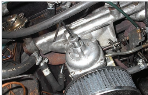
Tuning the carbs, adjusting the mixture
