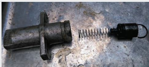
Stripping down the slave cylinder during overhaul
