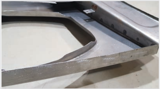
New Panel - Holes & Supports are missing - Templates will be Supplied
