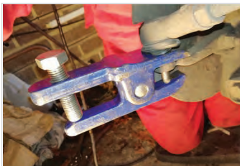
Breaking the Track Rod End Taper Joint with a ball joint splitter
