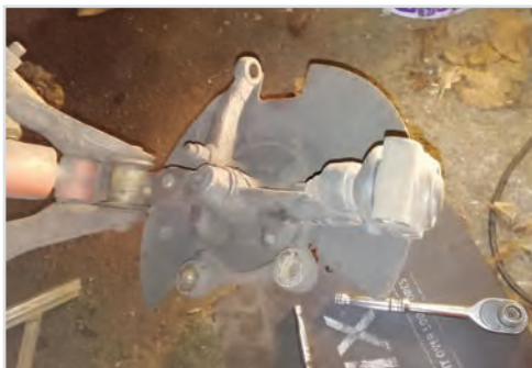
Upper Ball Joint and Vertical Link Assembly Free at the top.
