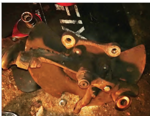
Removing the Trunnion to Lower Wishbone Bolt.
