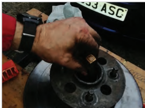
Drift out the Bearing Races from the Hub Assembly
