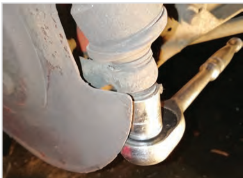
Removing the nut from the Track Rod End taper
