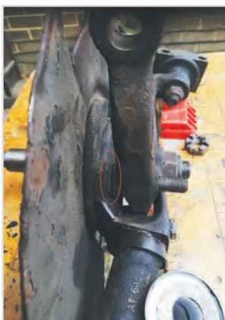
Drift out the Bearing Races from the Hub Assembly
