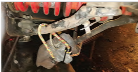
Supporting the Brake Calliper with a Bungee Cord
