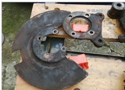
Disk Shield and Calliper Bracket Removed
