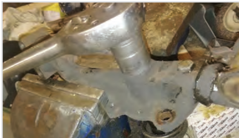
Removing the Stub Axle Nut.
