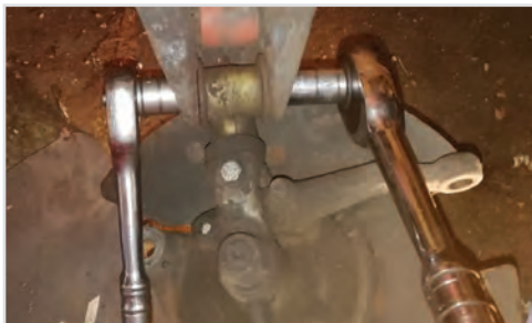
Removing the Trunnion to Lower Wishbone Bolt.
