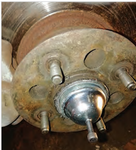
Removing the hub dust cap
