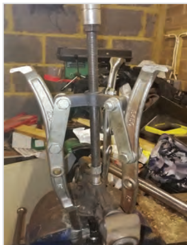
Trying to Release the Stub Axle with a 3 legged Puller
