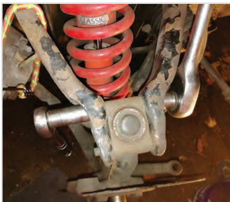
Removing the Fixings from the Upper Ball Joint to the Upper Wishbones
