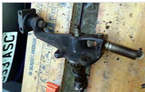
Trunion also unscrewed and ready to Remove the Stub Axle
