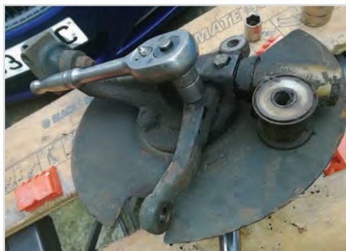
Disassembling the Vertical Link assembly
