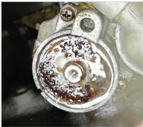
Serious Sediment caught by the gauze filter in the pump.
