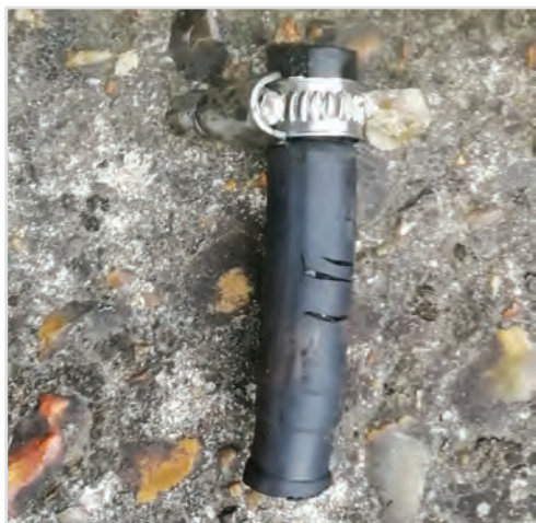
Supposedly Ethanol proof hose from eBay starting to break up.
