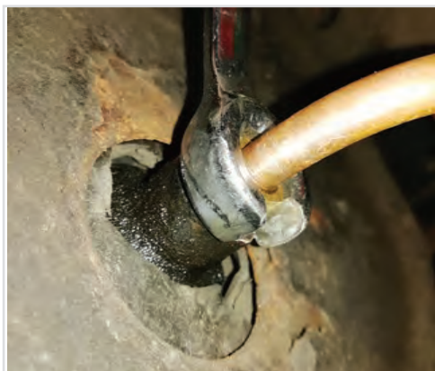
Using a brake pipe spanner to release the tube nut.
