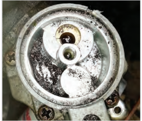
Sediment in the fuel pump body below the filter.
