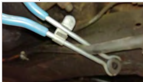
Using a hose clamp to seal the petrol hose.
