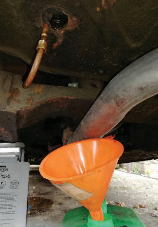
Outlet pipe removed and tank drained.
