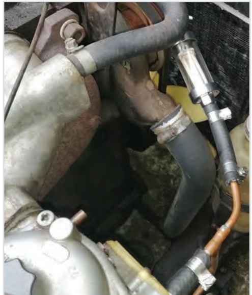
Inline filter before the carbs, note the new hoses and clips fitted.
