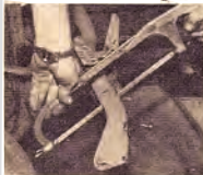
FRAME extensions are sawn off 2 in. from supports. Cover ends with something like metal cap or a plug
