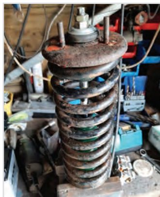
New shock absorber fitted - shame I did not have any nice shiny new springs!
