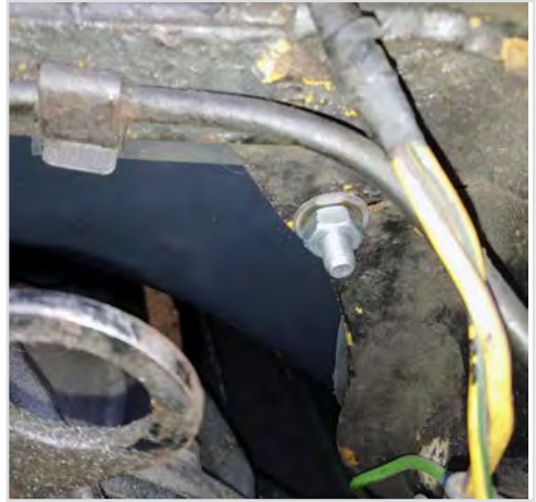
An upper front fixing nut and washer from the engine bay side.
