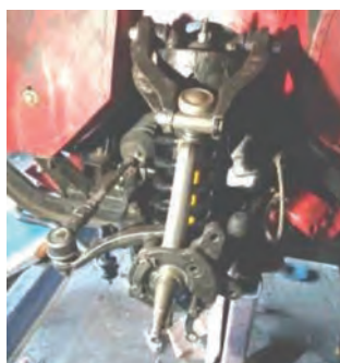
New NS vertical link and top ball joint
