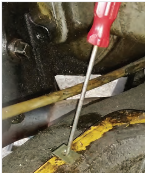
Aligning up a Spire Clip with a fixing hole in the bodywork.
