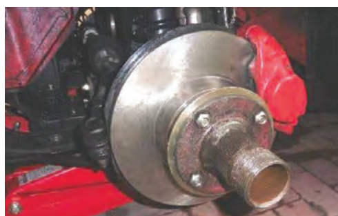
New hub and brake disc installed
