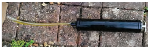
Gearbox filling Syringe pump.
