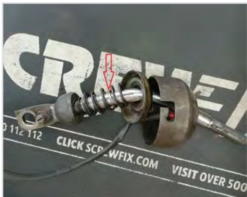
Circlip out of place.
