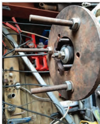
Spring compressed and top nuts on shock absorber.
