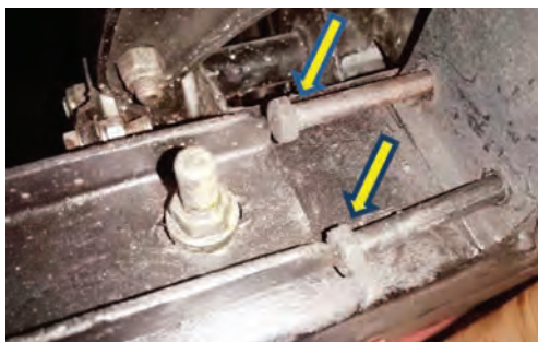
Bump stop bolts installed wrong way round
