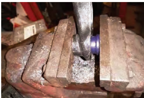
Fitting upper wishbone poly bush
