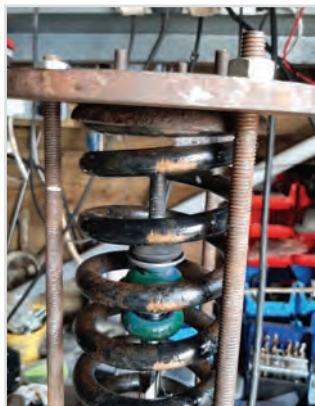
New shock absorber in position - you can see how much the spring needs to be compressed to allow the nuts to be fitted.
