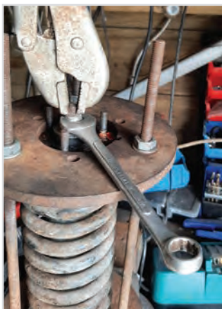
Spring and Shock absorber in spring compressor, compressed to allow nut to be removed, need to hold the centre shaft to stop it turning.
