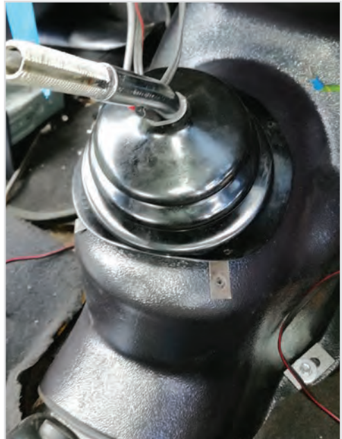
Gaiter being slipped over the gear lever.
