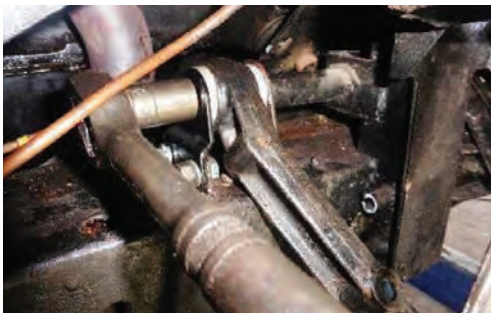
Lower inner wishbone bushes being fitted
