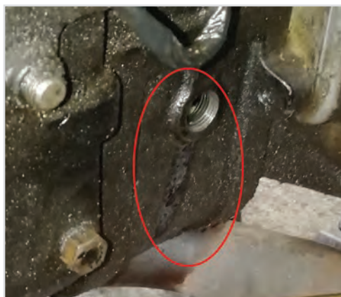
Oil leaking out of the filler hole means it's fully topped up.
