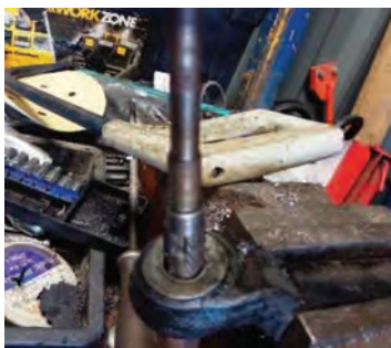
Pressing out NS stub axle from vertical link
