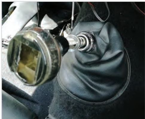
Gear Knob being refitted.
