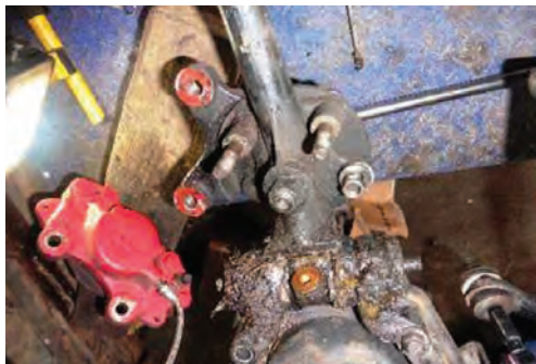
Old OS trunnion with vertical link attached
