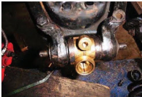
OS trunnion showing threads for vertical link
