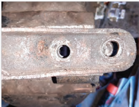
The end of the wishbone where the wear in the outer hole can clearly be seen.
