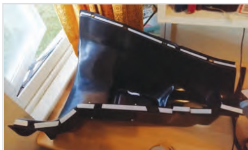
double sided tape fixed ready to accept the seals
