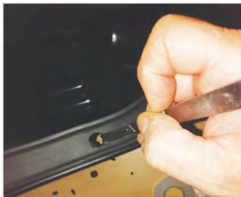
Cutting the seal at the fixing hole position
