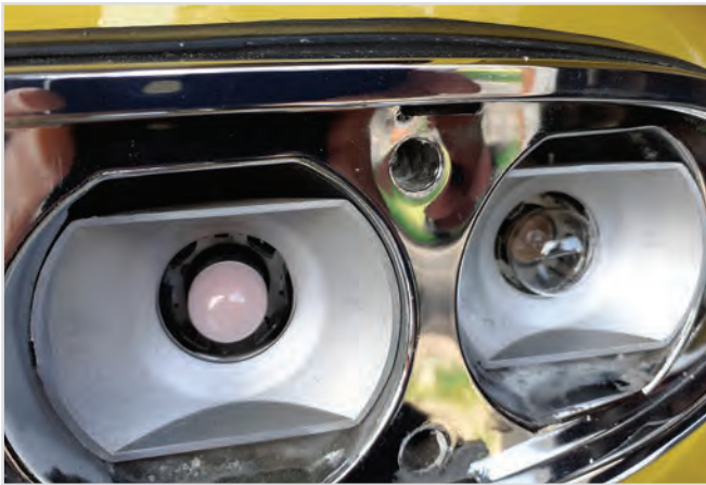
Pic 3. Indicator and brake/sidelight 'reflectors'
