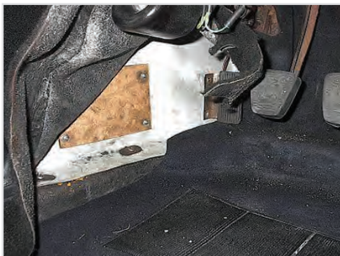
Hatch to access the gearbox oil filler in my original gearbox tunnel.
