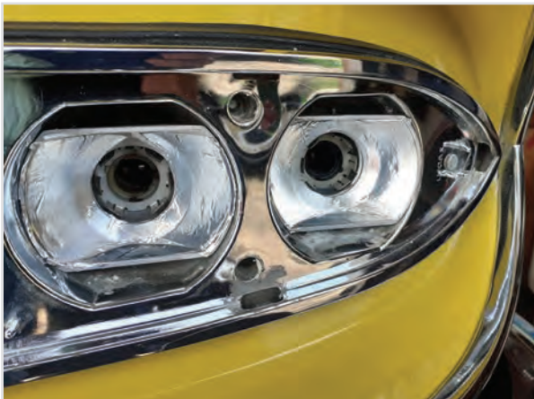
Pic 4. Aluminium tape applied to surfaces
