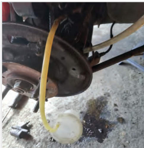
Using a brake bleeding kit to catch leaking fluid once pipe disconnected.
