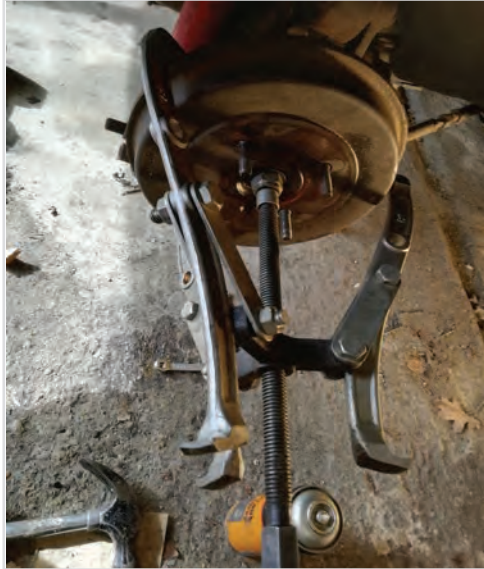
Using a 3 legged puller on the drum
