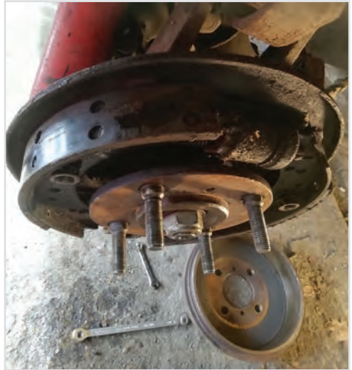
Brake assembly with drum removed (LH).
