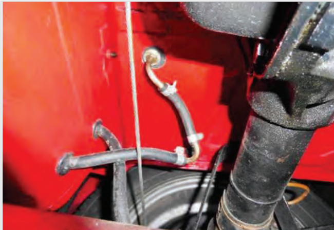
Pic 1 - Existing fuel tank set up under boot
