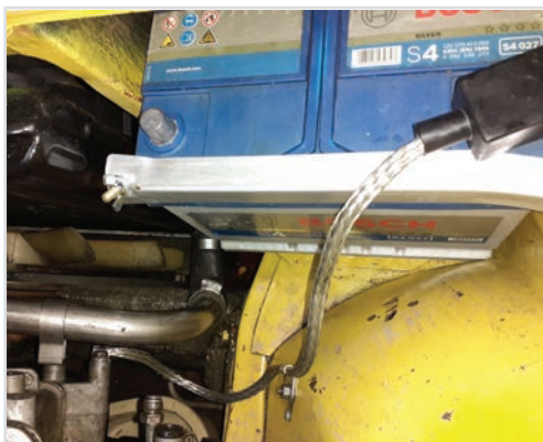
Pic 6. New engine to body to battery earth cable fitted
