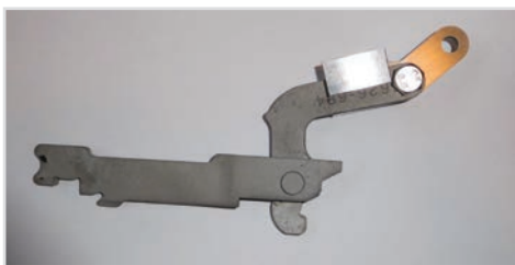
Pic 7. Tony Hart handbrake improver as fitted to lever
