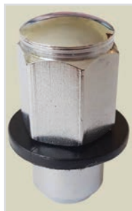
Special wheel nuts used for Mk3 GT6s to secure the centre hub caps.
