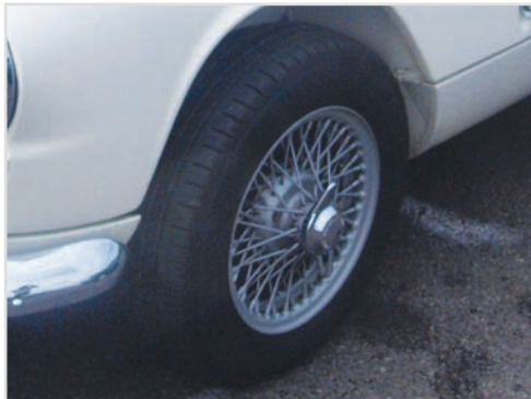
Spline fitment wire wheels with eared spinners as fitted as a factory option to early MK1 GT6s
