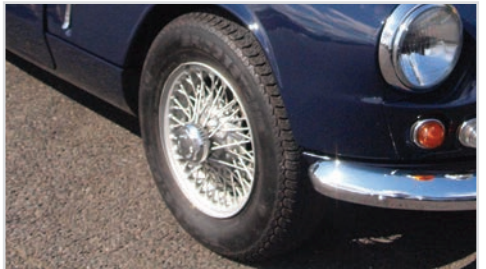
Spline fitment wire wheels with hex spinners as fitted as a factory option to late MK1 and MK2 GT6s
