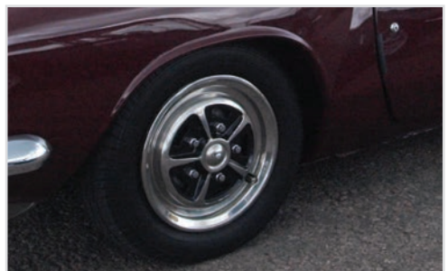
GT6 MK2 with Rostyle style hubcaps, the 5 wheel nuts on the hubcaps are dummy ones, underneath the wheel is held on with the standard Triumph 4 x 3/8 unf wheel nuts on a 3 3/4 inch (95.25mm) PCD.
