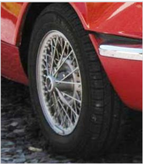
Bolt on Wire wheels as fitted to Mk3 GT6s as a factory option.
