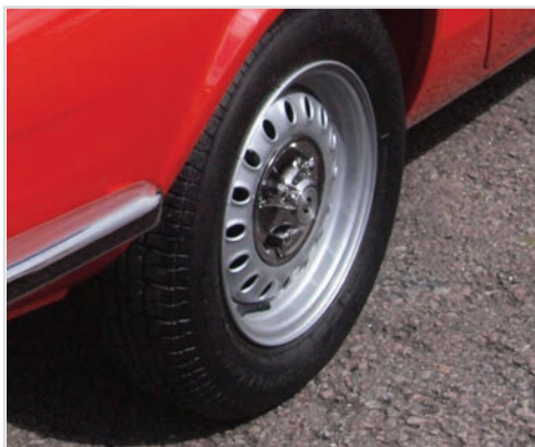
GT6 MK3 standard 4.5J Dunlop oval holed wheels.
