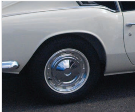
GT6 MK1 Standard steel Wheels with slotted Chrome Hub Caps
