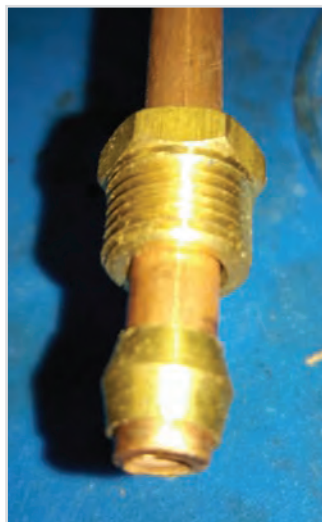
Olive and Tube Nut arrangement on 1/4" copper fuel pipe.
