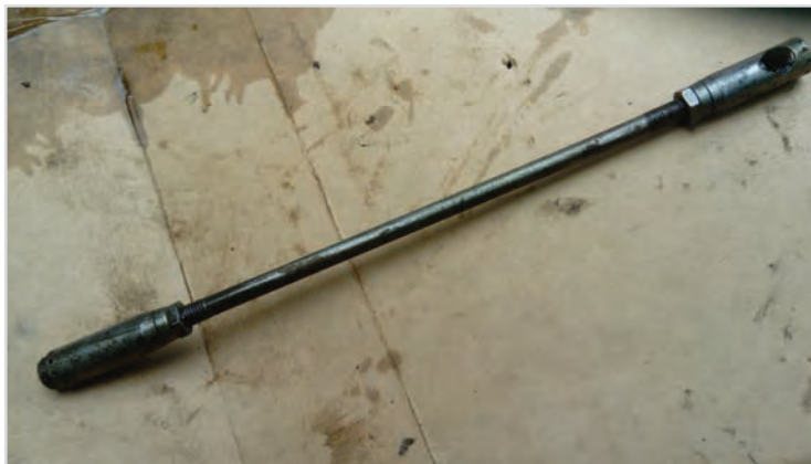
Main link rod too long even after making full adjustment
