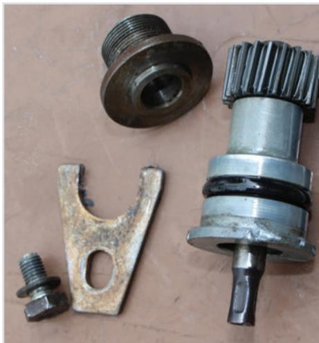
**Pic.2. J-type speedo driven gear Assy.**
