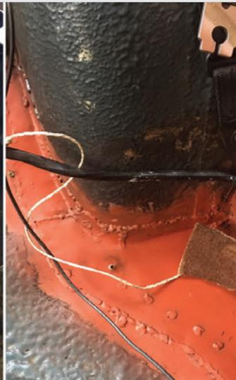
helped him prepare the 2000 ready for the new metal whilst I was at work. By the end of the bank holiday the new metal work was neatly fabricated and welded into place. Grateful to Nigel for his assistance, the 2000 was delivered straight to the MOT garage which she passed with an advisory on the
