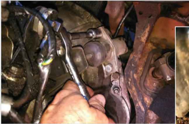
Unbolting the Slave Cylinder
