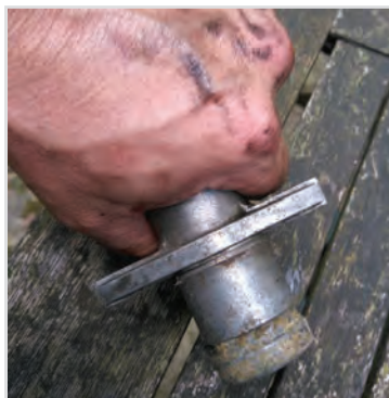
Tapping the piston assembly out on a bench
