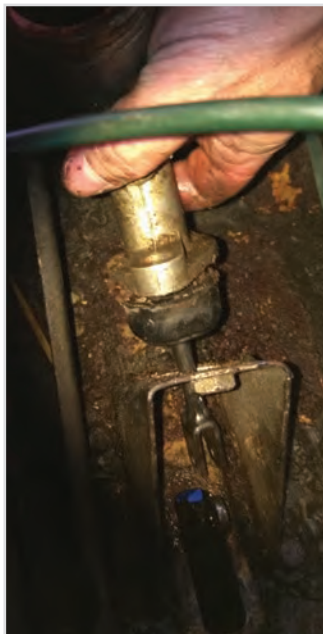
Master Cylinder being removed
