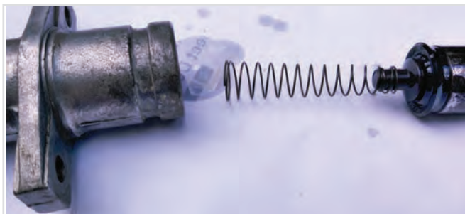
Ready for re-assembly of the piston back into the cylinder after fitting a new seal.
