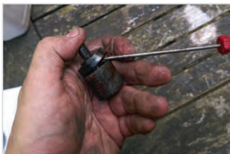
Removing the old worn seal
