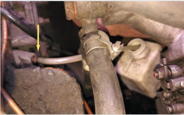
Pumping out the fluid via the bleed nipple.
