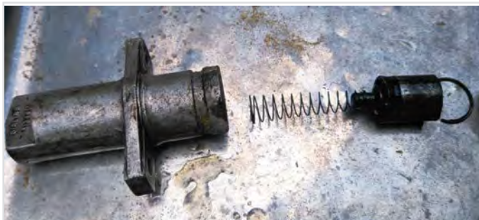
Inner piston assembly removed, complete with return spring.
