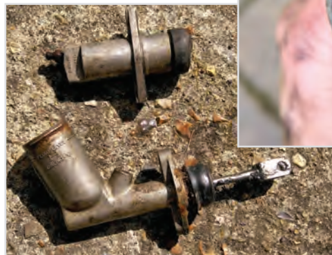
Master and Slave removed ready for rebuilding
