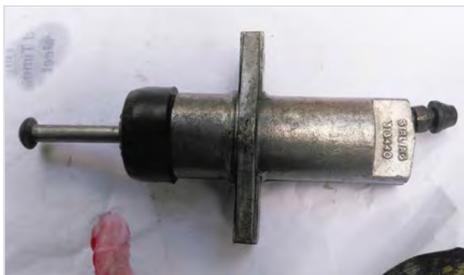
Rebuilt Clutch Slave cylinder unit.
