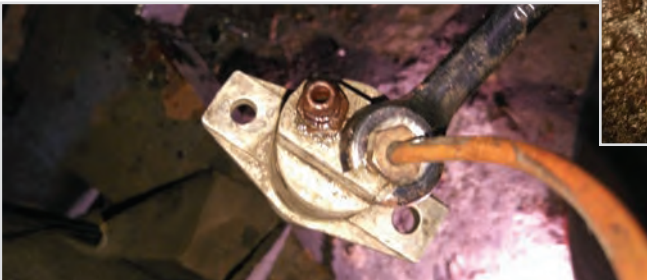
removing the hydraulic pipe from the slave using a 7/16" flare ring spanner.
