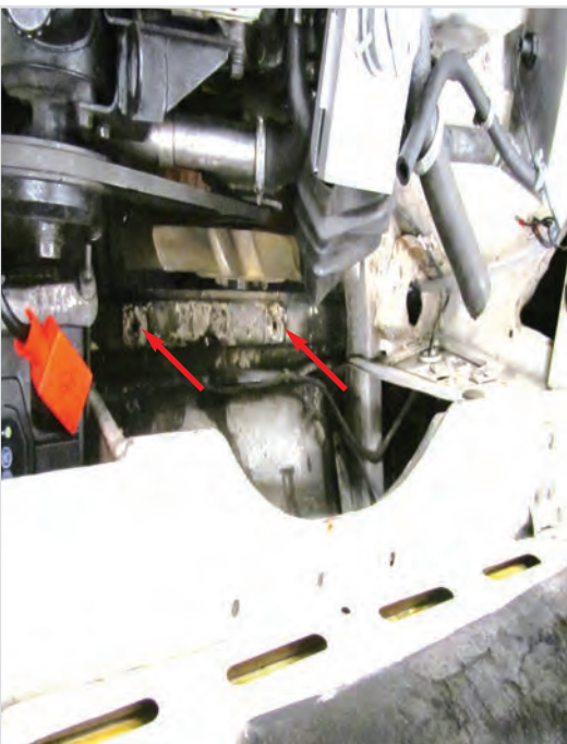
Figure 2. radiator removed showing where the bottom of the radiator mounts to.
