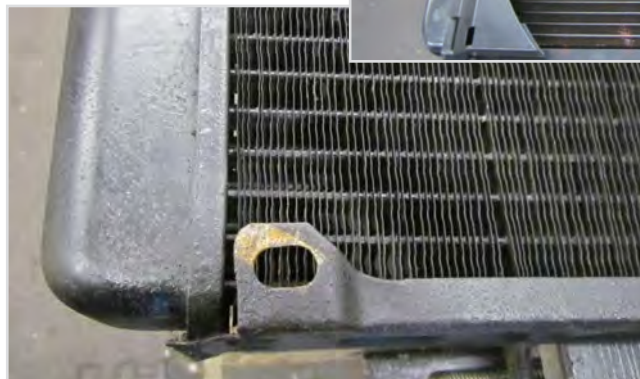
Figure 6. Shroud mounts on original radiator
