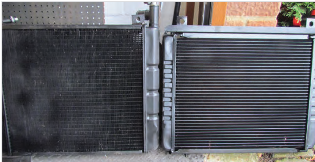
Figure 1. Standard Rad (Mk2) on the left and Supergill on the right.
