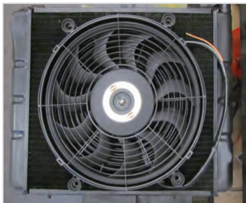
Figure 3 Showing size of electric fan compared with radiator
