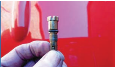
1. Mixture adjustment screw "O" ring
