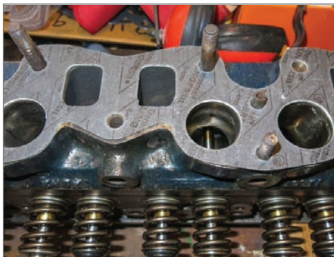
Picture 7 Moss Performance manifold gasket aligns better with the ports than a standard gasket
