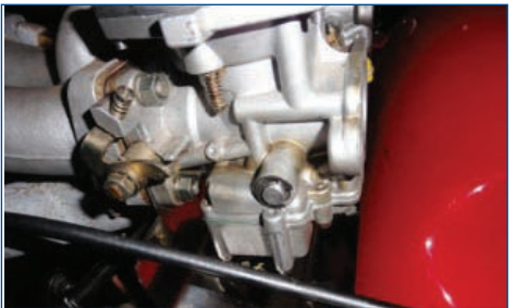
3. Rear carb cold start spindle
