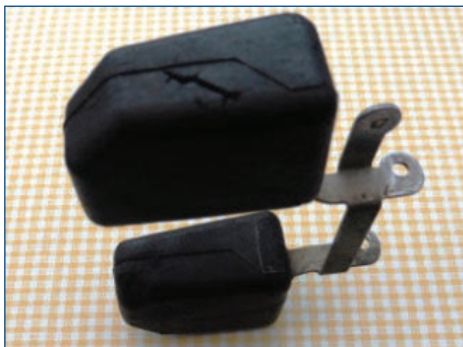
4. Crack in float
