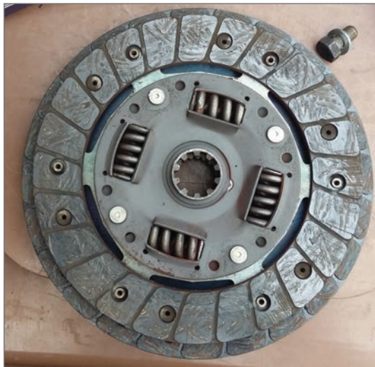
Pic 3: Old and new clutch plate (One on top of the other)
