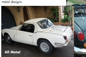
Some are bolted through the bootlid while others are held on by rubber suction feet with side clamps.
