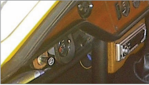
Picture 3 Cigar lighter socket fitted under the dash on my GT6
