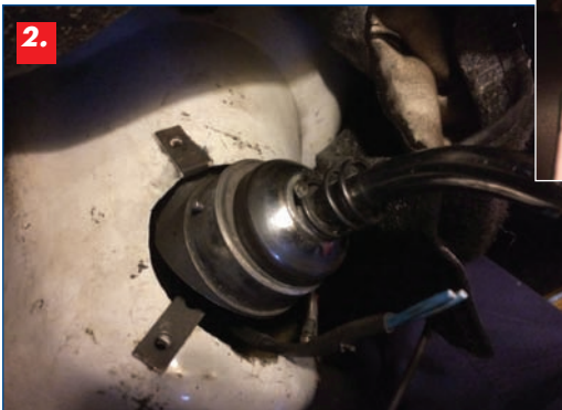
Picture 2 & 3 The anti-rattle spring had punched it's way through the Nylon Dome washer
