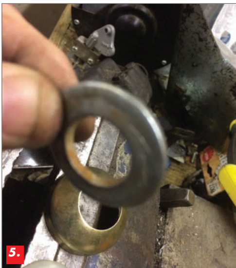
Picture 5 I found a suitable steel domed washer.
