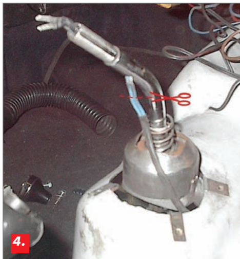
Picture 4 I had to cut the overdrive switch wires here to remove the anti-rattle assembly
