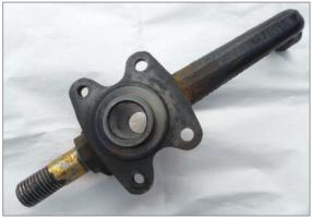
new 'surprises' – this month was a front vertical link that has been brazed back together after the typical snap at the top of the thread.
