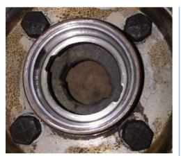
Photograph 4 Recesses clearly seen with bearings removed
