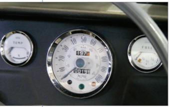
The dashboard layout was unique to the car featuring three dials, a white central speedometer reading to 100 mph flanked by temperature and fuel gauges.
