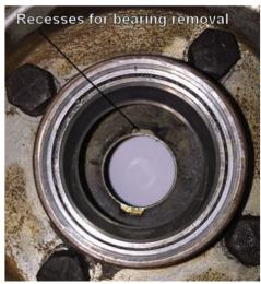
Photograph 3 Recesses in hub for bearing removal
