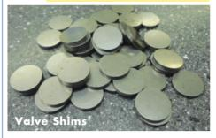
Intake valve clearance should be 0.008", exhaust 0.018".
