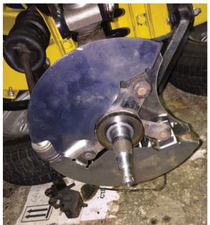
Photograph 1, Stub axle cleaned and ready. The bearing spacer and outer cover are not very clear on diagrams.
