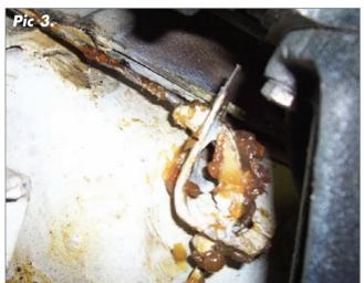
and including the 2 Litre (Mk1). However, with the introduction of the Rotoflex rear suspension on the Mk 2 models the cable guides were shifted from the chassis to the body tub, Picture 3, to enable the cable to clear the rotoflex rubber doughnut couplers on the rear
