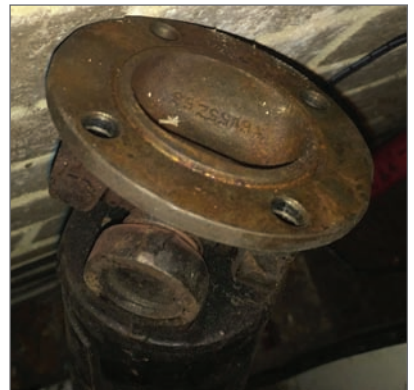
Picture 5 Old prop flange has a bowl shaped recess for clearance
