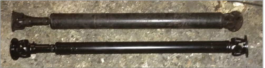
Picture 2 Old and new props, note the thinner tube on the new one.
