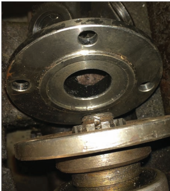
Picture 6 New prop flange has a smaller hole for clearance
