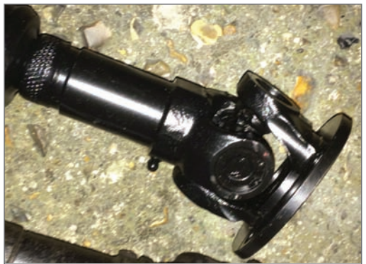
Picture 4 New Prop with grease nipples in place.
