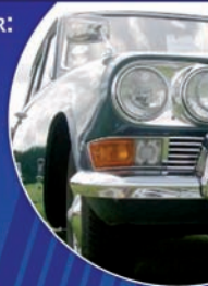
Front wheels still extend beyond the arches despite losing 5mm each side!
