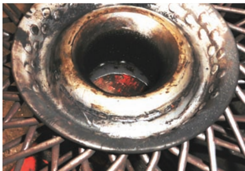
Evidence of wheel studs digging into inner face of road wheel
