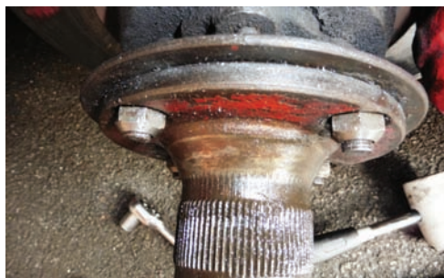
Cause of the damage - the studs are too long
