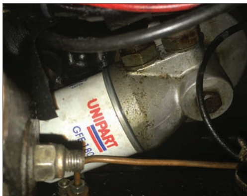
Picture 4 Spin on adaptor oil cooler take off
