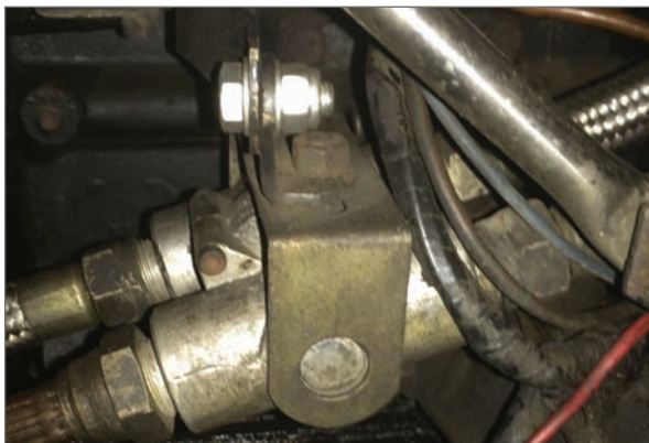
Picture 2 Oil Cooler Thermostat
