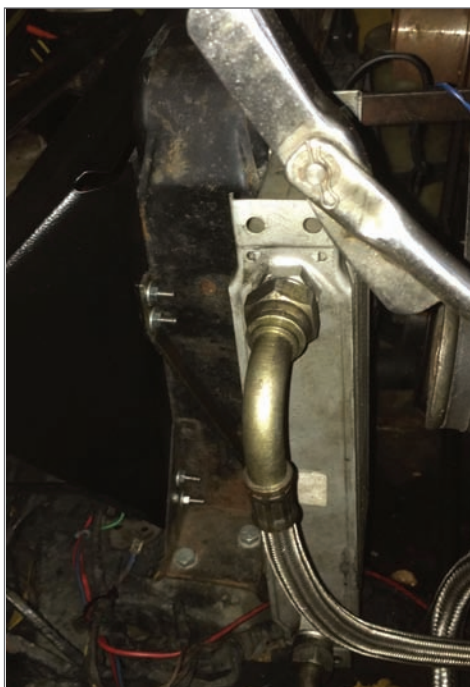
Picture 3 Oil Cooler at Side of Radiator
