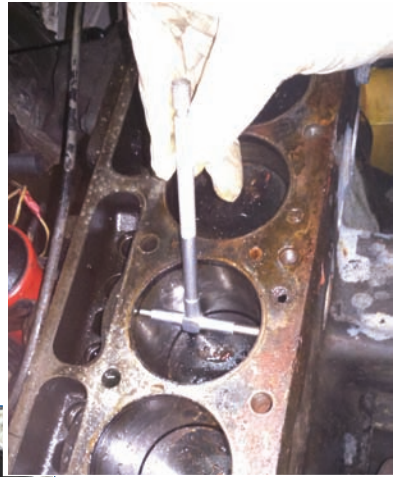
Measuring Bores with tele gauge
