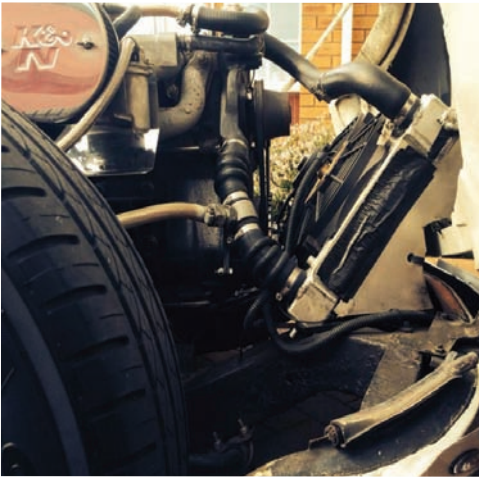
Picture 6 Golf Radiator in place fitted at an angle
