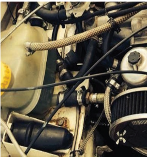
Picture 7 Expansion bottle mounted next to Clutch Master Cylinder
