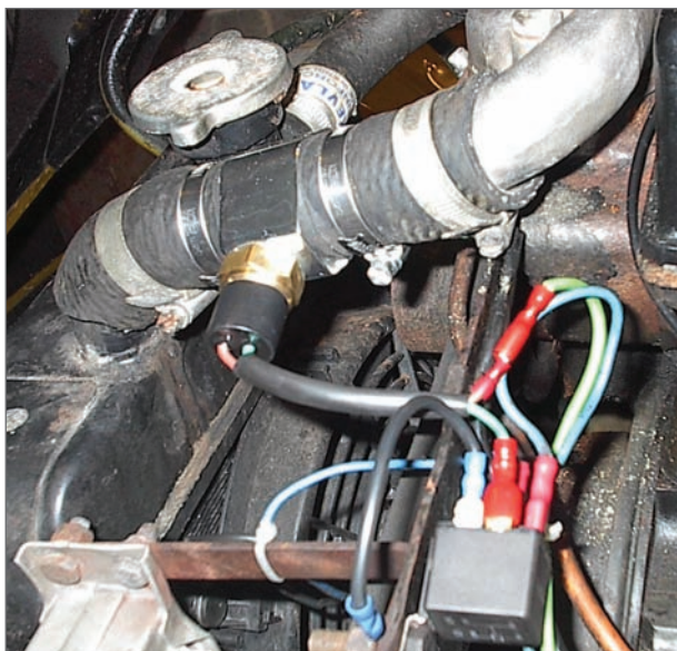
Picture 1 Billet alloy housing with modern fan thermostatic switch.
