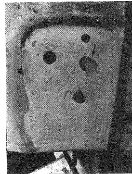
Fig. 2 Underside of bodyshell with rotted through outer skin near to mounting point bolt holes
