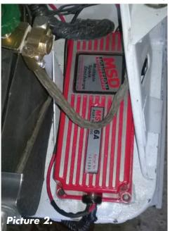
and the A post support, this is a good location as it is close to the fuse box and the earth strap location. Picture 2.
