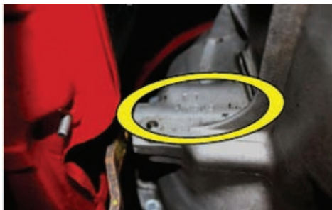
TR4 gearbox serial number
