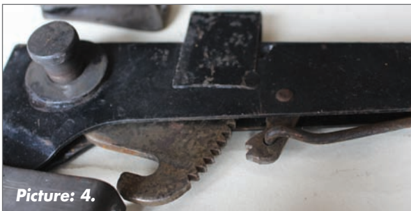
Picture 4: Close up of the early Spitfire ratchet and pawl.
