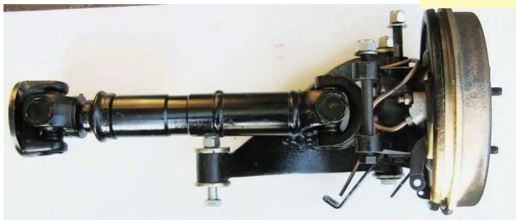
Picture 2 The Kingston Sportscars version of the solution. Looks like a Tubular rather than solid drive shaft a bit like a propshaft.
