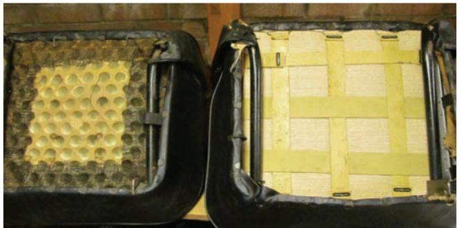
L/H seat as original minus the rubber support. R/H seat repaired with new sponge and a piece of hessian backed carpet with strong elasticated webbing support.
