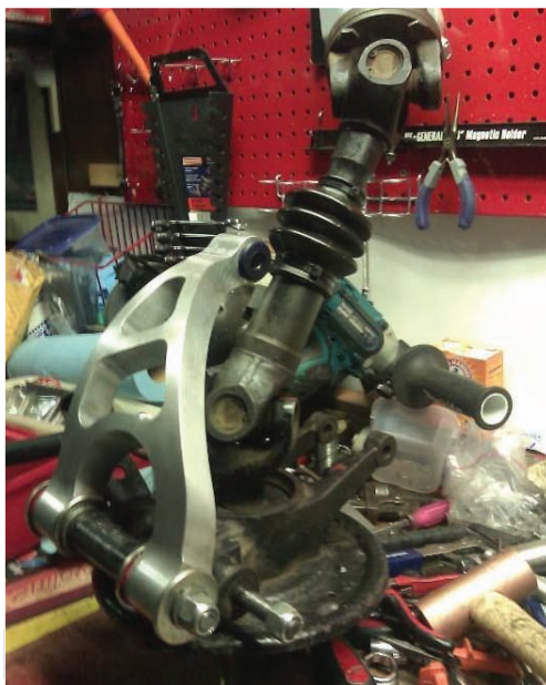
Picture 1 Leon Guyot's UJ/Sliding joint rear driveshaft set up on his Vitesse, note also the rather nice alloy bottom wishbone!
