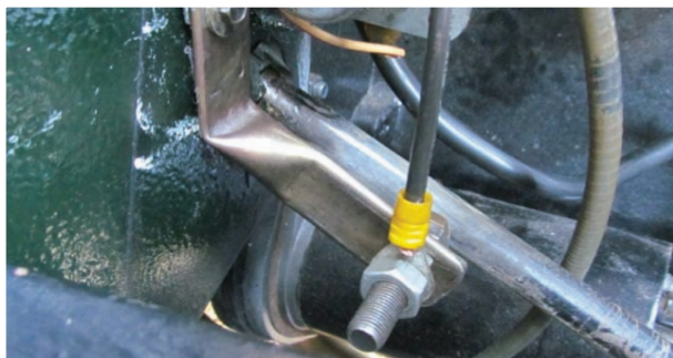
Earth wire taken directly from the battery to a sprung loaded plunger which contacted directly onto the steering column.
