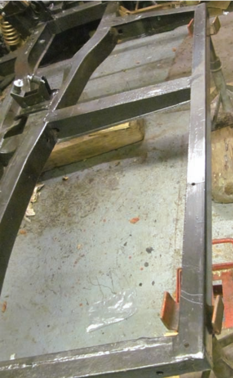
Chassis cleaned and painted with new outer side rails fitted.
