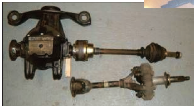
Picture 3 The "Bowler/Jones" set up compared to a standard Rotoflex Driveshaft. Picture was downloaded from a listing of a set that came up on ebay recently so apologies for the poor
