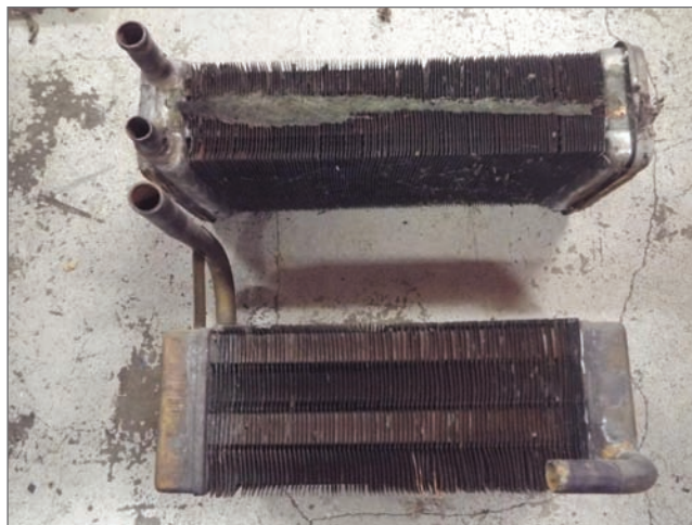
Pic 2. Heater matrix - Smiths top Delaney & Gallay (slightly deeper) bottom
