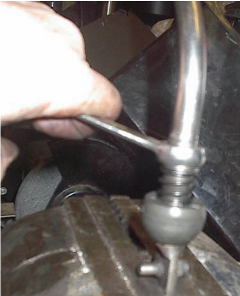
Picture 22 A little tip for refitting the Spring Clip holding the Inner Spring in place Use a ring spanner over the gear lever shaft as this makes the job really easy!
