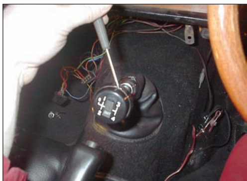
Picture 6 Remove the Knob Top and Switch assembly.
