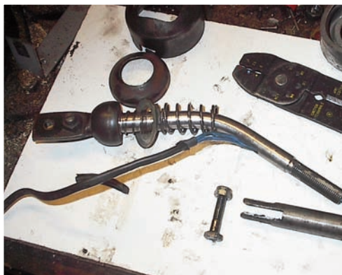
Picture 18. Remove the Bayonet Shroud, Inner Metal Shroud, Plastic Shroud and Outer Spring from the Gearlever.
