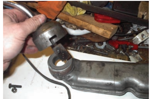
Picture 16. Remove the Gearlever held in place with a bayonet type fitting.
