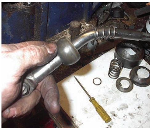
Picture 20. Next remove the spring and then the Plastic Ball Bush.
