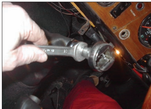
Picture 7 Slackening the Chrome Tapered Lock Nut under the Knob.
