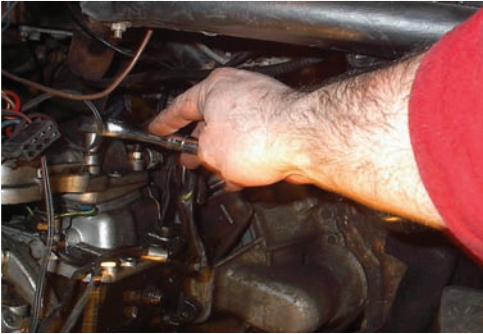
Picture 12. Removing the Remote Extension assembly fixings from the top of the gearbox.
