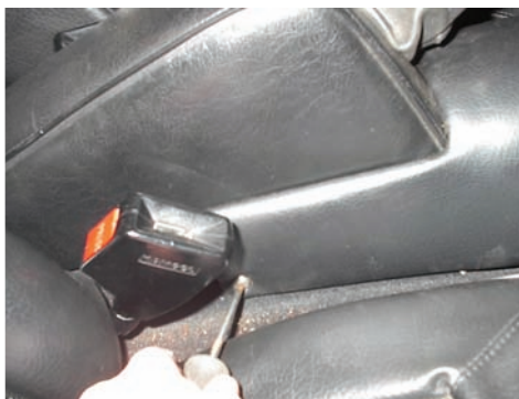
Picture 2. Removing the Trim under the handbrake.
