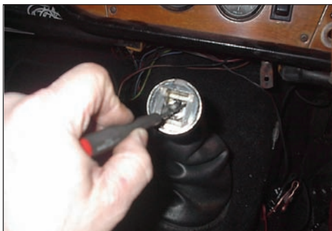
Picture 8. Unscrewing the nut within the Knob chamber.
