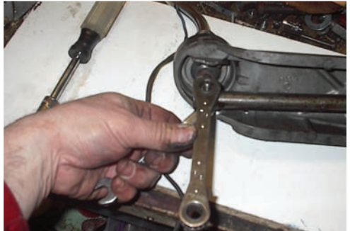
Picture 15. Undo the nut and bolt holding the bottom of the Gearlever to the Remote Shaft
