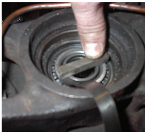
Measuring the set up with shims and distance piece to check
