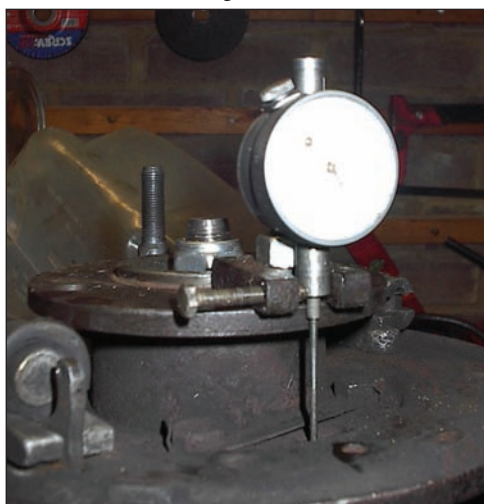
Checking the end float with a dial gauge
