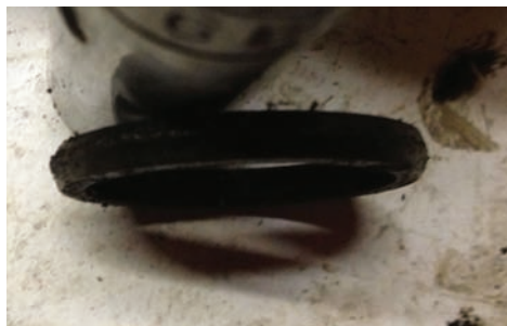
Damaged distance piece, this should have a straight outside edge rather than tapers.
