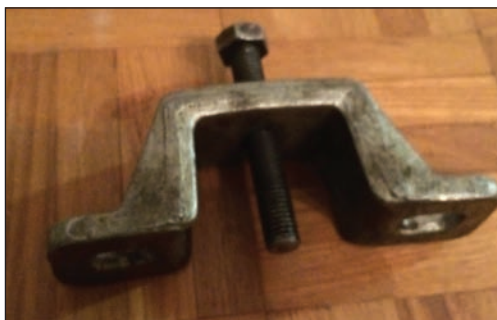
A light duty hub puller like this should be adequate to extract a Rotoflex hub.
