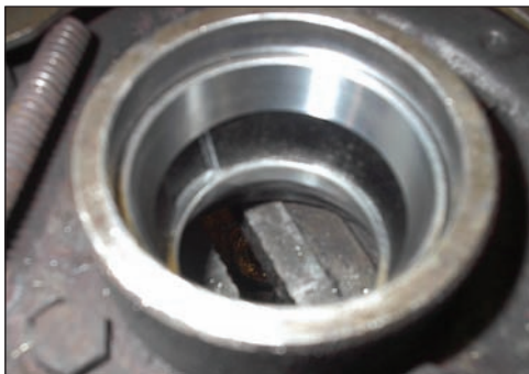
Bearing race for the outer hub bearing drifted into place in the vertical link.
