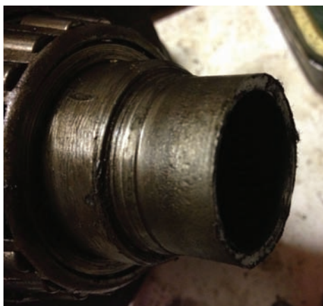
Damaged Hub and distance piece due to leaving a worn bearing for too long!
