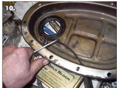
Photo 10 Hook to pull tensioner into place whilst fitting cover.
