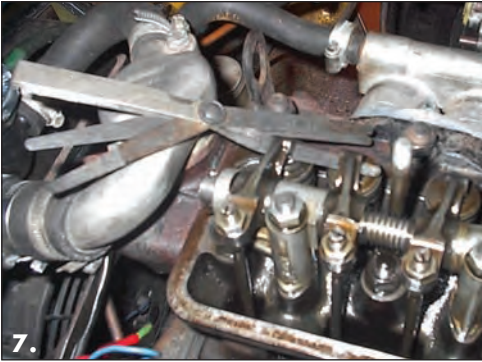
Photo 7 camshaft for both valves of No 1 cylinder at an equal clearance, ie the rocking point.
