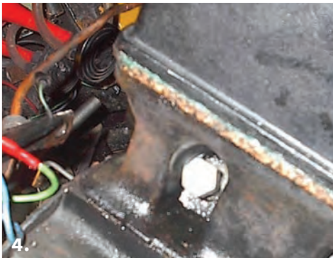
Photo 4 BMW Mini wheel bolt screwed into the plug hole of No 1 cylinder.
