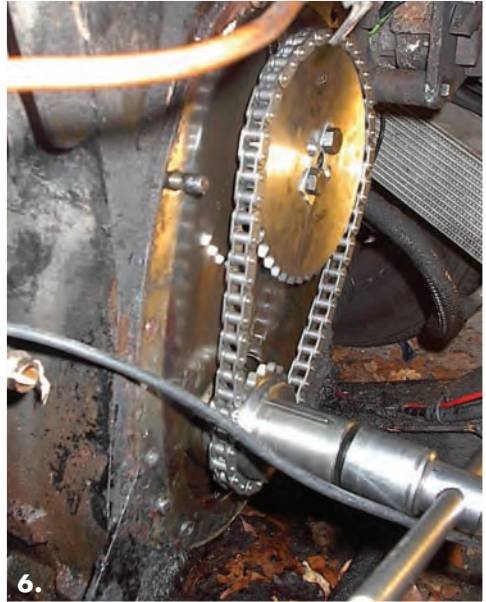
Photo 6 Camshaft sprocket in place, note the woodruff key
