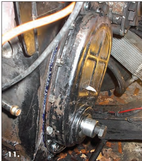
Photo 11 cover fitted with Blue Hylomar sealant to help keep it oil tight.
