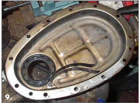
Photo 9 New oil seal and tensioner fitted
