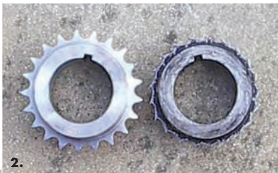
Photo 2 Timing chain sprocket had lost it's teeth, here's the old one and the replacement.
