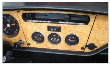
did to locate the gauge where the light switch is originally located, and move the light switch. Others use a mounting plate as in the photograph.
