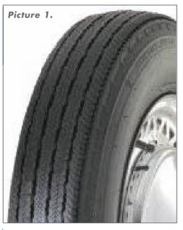
the greater weight of the Vitesse or to improve the road holding that made Standard Triumph fit the wider tyres to the 1600? I can only hazard a guess that it may well have been a bit of both. The wider tyres also brought other considerations as though the Vitesse 6 has the same differential ratio as the Herald 1200 because it is fitted with wider tyres this makes it slightly higher geared. The figures are 15.7mph/1000rpm for the Herald 1200 and 16.4mph/1000rpm for Vitesse 6.
