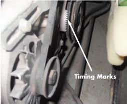
centre using the timing marks found on the crank front pulley
