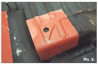
The best I could find was a rear corner repair section (pic 5), but there are no complete floor pans as in the GT6 or Spitfire.
