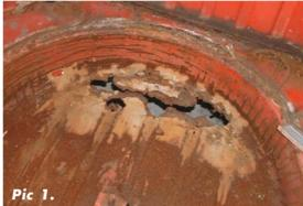
These are often the most serious areas to go, where moisture soaking in carpets and underlay eats its' way through over the years, and often the hardest areas for which to find repair sections.
