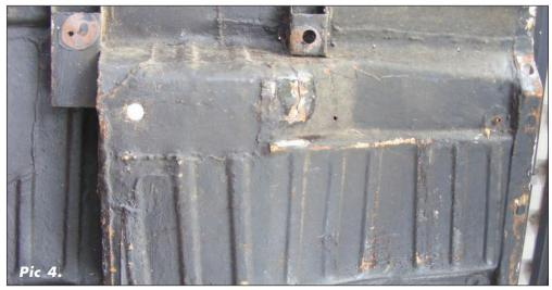
The repair panels for under the rear seats have always been available, with the kidney - shaped dimple and the drain hole. Quality does vary so shop around (pic 6).
